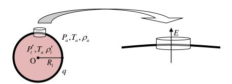
E = electric field on the film surface that results from all other parts of the soap film, excluding the surface inside the pill box itself.
