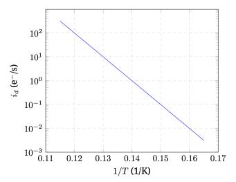
The graph shows how dark current varies with temperature. The units for dark current,  $e^{-}/s$  should be thought of as counting a number of electrons per second.
