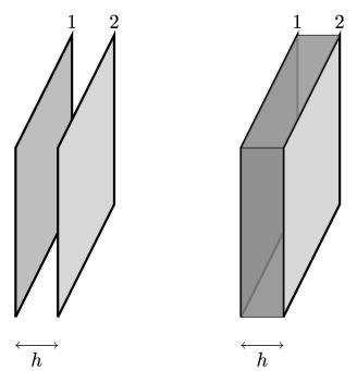
On the left is a simple model of two adjacent sheets 1 and 2 separated by a distance h. The sheets are not connected, and the perimeter is open to space. Assume the sheets are parallel. Thermal radiation can be exchanged between the sheets, and thermal radiation can escape through the perimeter gap. On the right, the perimeter gap has been shaded to help visualize.
