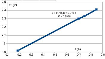
The regression line slope gives directly  $R_s \approx 0.75 \,\Omega$ .
