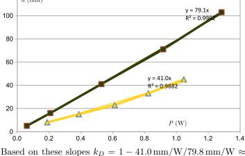
Based on these slopes  $k_D = 1 - 41.0 \text{ mm/W}/79.8 \text{ mm/W} \approx 0.48$
