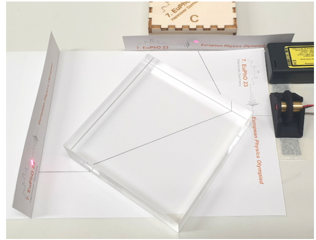
Figure 16: Determination of the laser polarization using Brewster reflection. The reflected beam will vanish at horizontal polarization.
